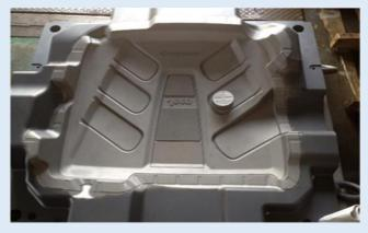
Textured surfaces require protection. The peaks of the textured surfaces are the first areas of mold detail to experience wear.
