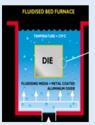
The DYNA-BLUE® process is not a line of sight process as the fluidized bed particles carry the DYNA-BLUE® process uniformly thru holes, bores, ribs, even thru the water lines to provide corrosion resistance.
