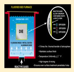
Wear tests have shown that the DYNA-BRITE™ process resists wear and corrosion better than lon/Gas Nitride, Chrome, Nickel and other coatings due to the hard wear resistant compound layer (75+ HRC) which is supported by a nitrogen rich diffusion layer (65 HRC).
